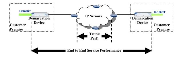
Delivering intelligent Ethernet services requires a network architecture that can support both robust service delivery and verification of SLAs. Customer premise
